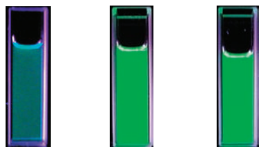
Figure 2. Fluorescence of naphthacene (left), 2a (middle), and 2b (right) in hexane at room temperature. The concentrations of the solutions of naphthacene, 2a , and 2b are 1.2 \times 10^{-5} , 1.0 \times 10^{-5} , and 1.1 \times 10^{-5} mol dm ^{-3} , respectively. Excitation was carried out with a low-pressure mercury lamp.
